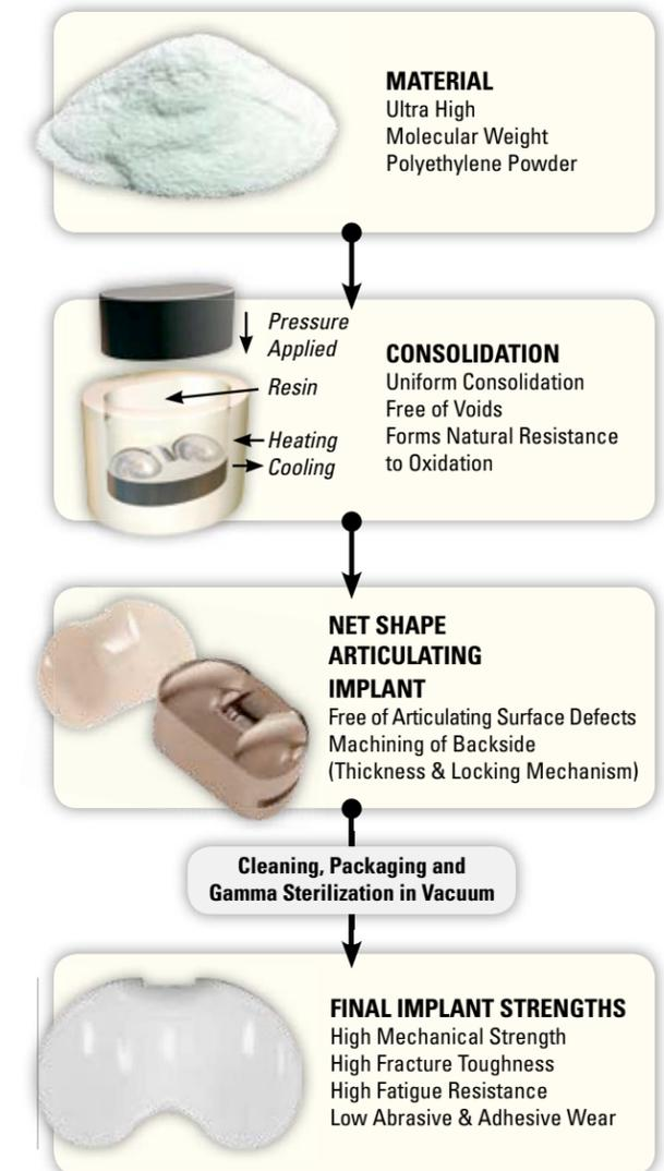
FIGURE 12: Manufacturing Process for NCM Polyethylene Inserts
