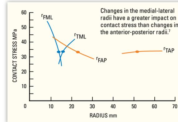
Figure 3b: Optimum Congruency for Minimizing Contact Stress
