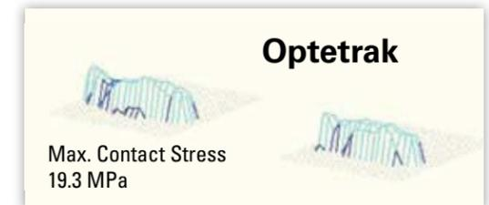
Figure 4: Optetrak Demonstrates Lower Contact Stress
